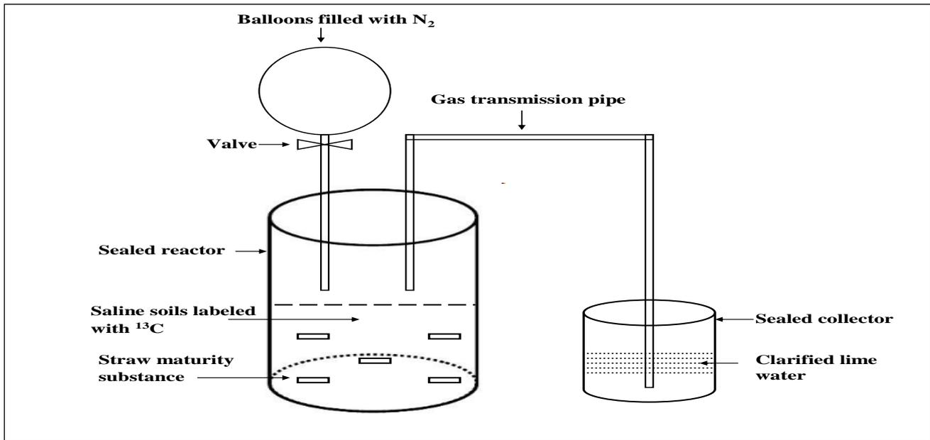
**Figure 1:** Introduction to test apparatus
